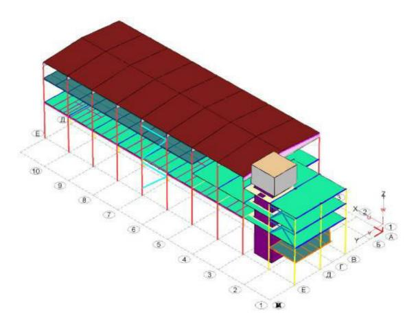
**Figure 2 – Building calculation model**
