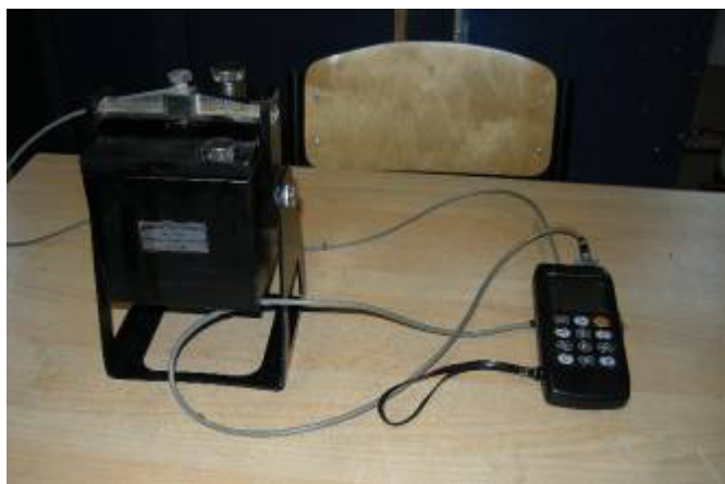
Figure 1 – Illustration of the dilatometer with the measuring electronic unit
