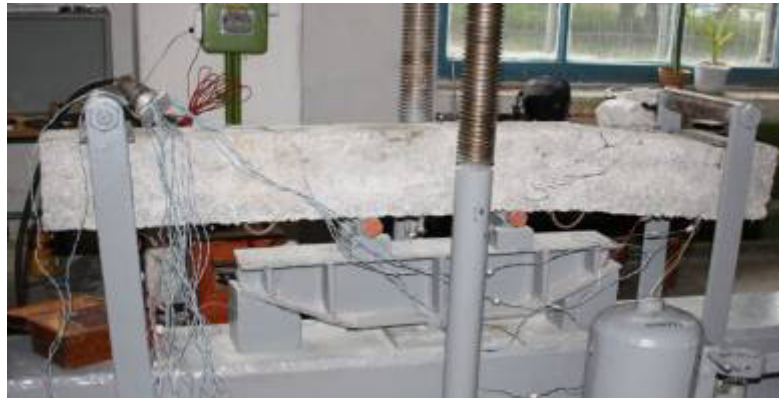
Figure 9 – Investigation of beam 1B – FC – 1 on flexure
