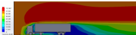
Figure 17 – Flow chart of the main train with a low cabin and ordinary ramp
