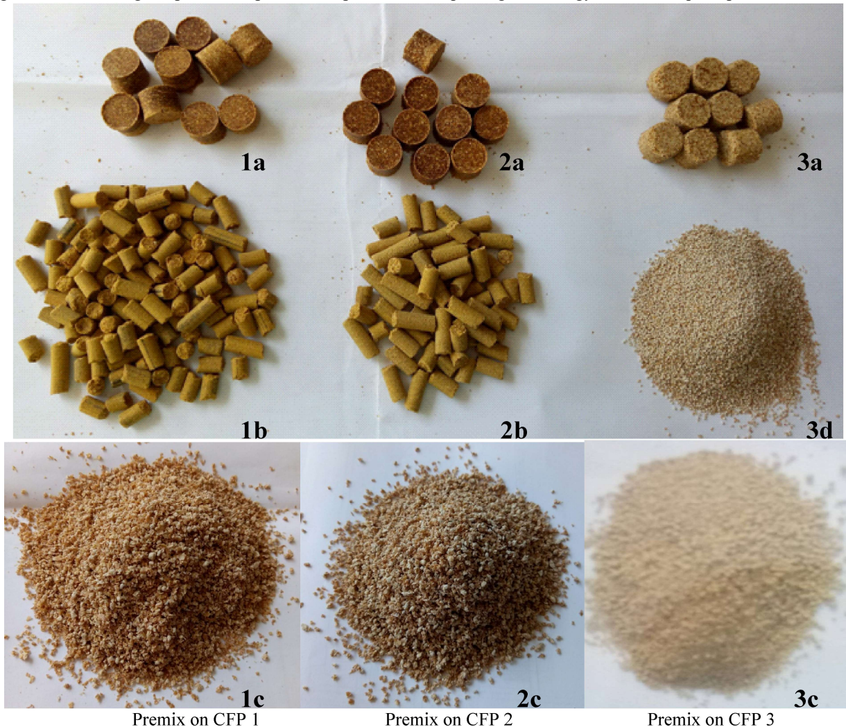
Fig. 5 - Premix obtained by the following methods: briquetting (a), granulation (b), cereals (c), rolling (d)
