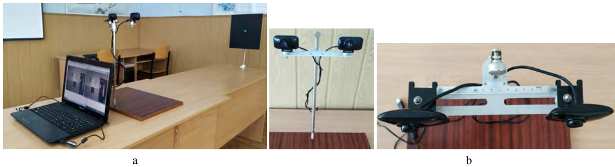
Fig. 4. General view of the laboratory stand – a; stereo pair design – b
