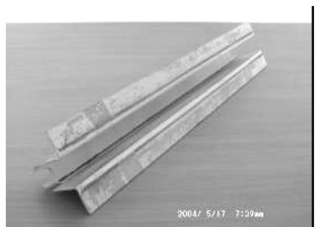
Fig. 7. Hot-formed parts
