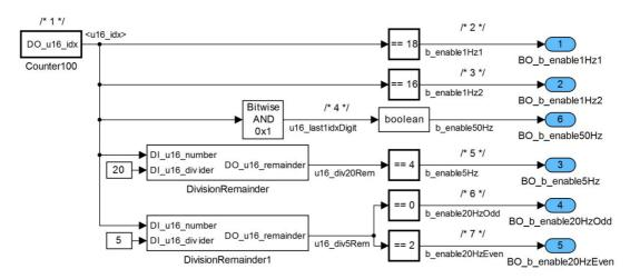
Figure 4. Trigger generating algorithm implemented in Simulink model
