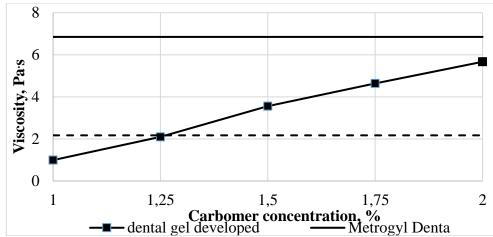
Fig. 2. The dependence of the structural viscosity of the dental gel at a shear rate of 41.6 s<sup>-1</sup> on the concentration of carbomer in comparison with reference drugs (at 25 °C)
