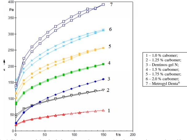
Fig. 1. Rheograms of dental gel, depending on the concentration of carbomer in comparison with reference preparations (at 25 °C)
