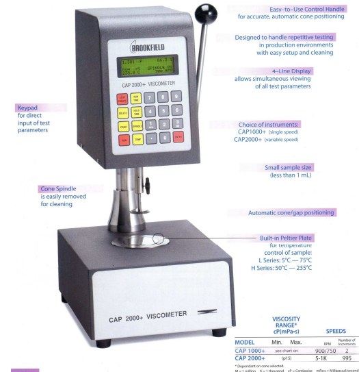
Fig. 2. Brookfield viscometer CAP2000+ and some its characteristics [9]
