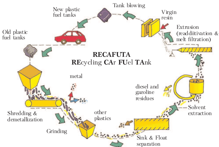
Figure 5. Recovery of thermoplastics within the fuel system (Solvay Company handouts)
