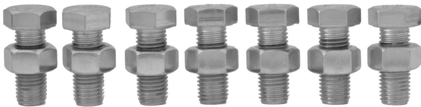
Figure 2. Some test samples after sealing with anaerobic adhesive (Authors' development)
