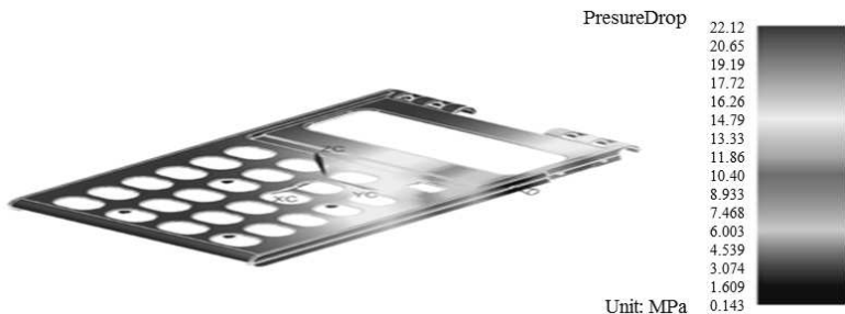
Figure 10. Pressure drop analysis
