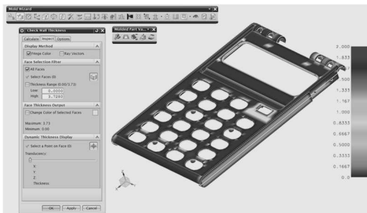
Figure 3. Results of the thickness validations
