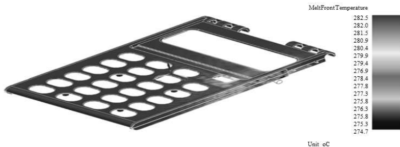
Figure 7. Melt front temperature analysis
