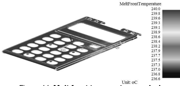
Figure 11. Melt front temperature analysis
