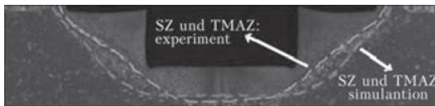
Figure 7. Comparison of experimentally and numerically determined thermo mechanical affected zone after FSSW of AA6082-T6 [11]
