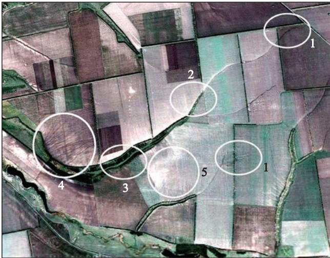
Fig. 2. Gully erosion manifestations from the high spatial resolution materials: 1-rain channels; 2-top cutting-in; 3-, 4-micro-gully erosion; 5-sheet erosion (satellite survey SPOT, spatial resolution – 5 m, April 2013)
