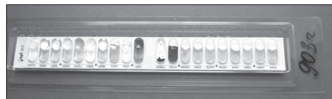
The general layout of API 20E test-system
