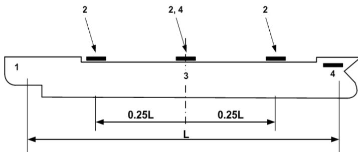
Fig. 1. The layout of the sensors of the ship's hull monitoring system recommended by the international maritime organization: 1 – ship's hull; 2 – strain sensors; 3 – midship; 4 – accelerometers;  $L$  – length of the vessel
