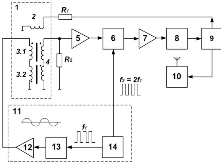
Fig. 3. A block diagram of a magnetometric channel
