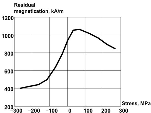
Fig. 2. The dependence of the residual magnetization from the tensile and compressive stresses in the elastic region for steel st3
