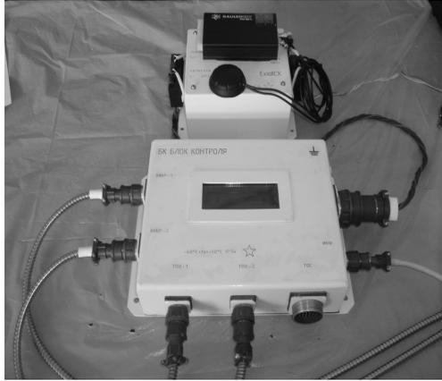
Fig. 6. Exterior view of the display unit of ship magnetic measuring complex
