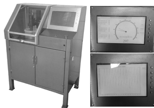
Fig. 1. Stand of verification of medium-speed diesels injectors state
