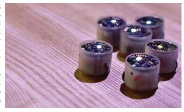
rechargeable battery, the touch sensor, a gyroscope, the optical sensor and the microcontroller. Capabilities of these microrobots are very far from capabilities of big ATLAS robots of the Boston Dynamics company, nevertheless, having united in group, they can carry out rather complex challenges.
