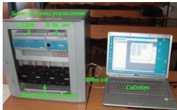
Fig. 2 – Appearance of the block of the robot control system by the manipulator "Electronics NC TM-01"
