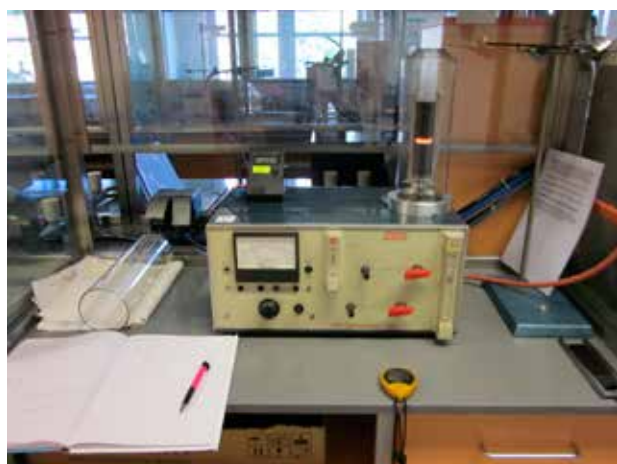
Fig. 1a. Apparatus for the determination of oxygen index at standard temperature Source: Own elaboration.
