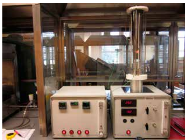
Fig. 1b. Apparatus for the determination of oxygen index at elevated temperature Source: Own elaboration.
