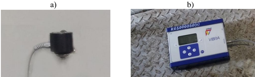
Fig. 8. The location and the sensor measurements of vibrations: a) location of the sensor on the tower wind turbine; b) sensor readings maximum displacements of the tower wind turbine
