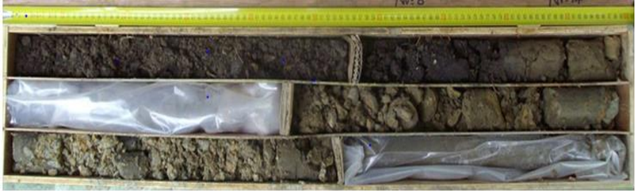
Fig. 2. Drilled coring in volcanic weathered basalt
