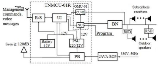
Figure 1 – Block Diagram of TNMCU-01R
