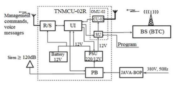
Figure 2 - Block Diagram of Radio-controlled TNMCU-02R
