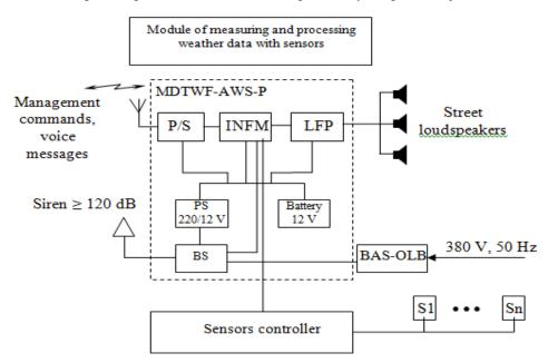
Figure 1 - Block diagram of radio-meteocomplex MCA-P
