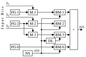
Figure 9 - "DISPERS" transmitter block diagram
