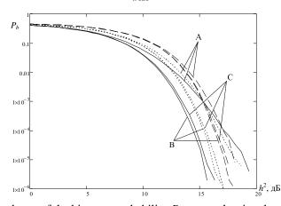
Figure 12 – The dependence of the bit error probability  $P_b$  versus the signal-to-noise ratio  $h^2$ : A - Gaussian distribution of useful signal; B – the binary distribution, C – symmetrized beta distribution where
