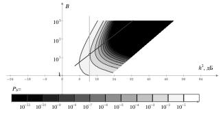
Figure 11 – Determining dependence  $B_{opt}$  on  $h^2$  for the DNSK
