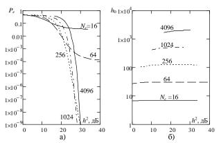
Figure 13 - The probability of synchronization errors (a) and optimal detector threshold level (b)
