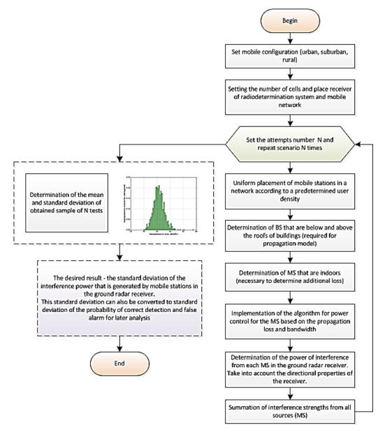
Figure 2 – Algorithm flowchart
