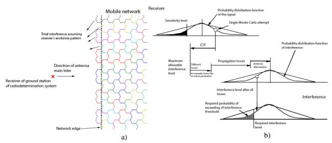
Figure 1 – Monte Carlo method to determine the effect of interference from subscriber stations mobile network
