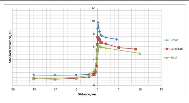
Figure 5 – Dependence of total interference SD from distance
