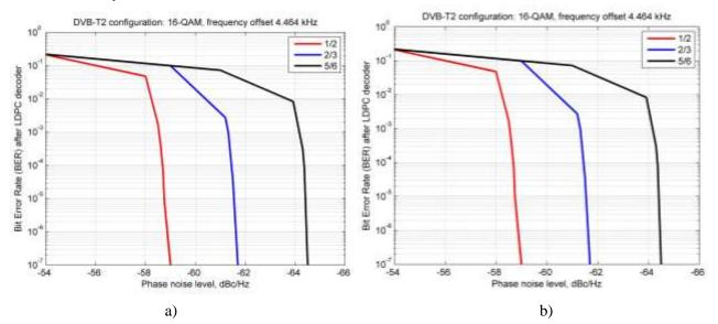
Figure 4 - Dependence of BER after LDPC decoder from phase noise level in DVB-T2 system for 16-QAM (a) and 256-QAM (b) modulations and 4.464 kHz frequency offset
