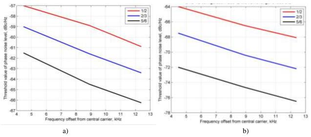
Figure 5 - Dependence of threshold level of phase noise from frequency offset for 16-QAM (a) and 64-QAM (b) modulations in DVB-T system
