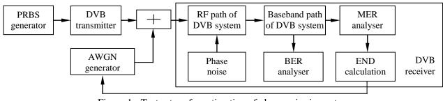
Figure 1 - Test set-up for estimation of phase noise impact on DVB-T and DVB-T2 system performance
