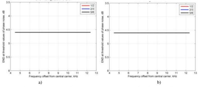
Figure 16 - Dependence of equivalent noise degradation value from frequency offset at presence of phase noise for 16-QAM (a) and 64-QAM (b) in DVB-T system
