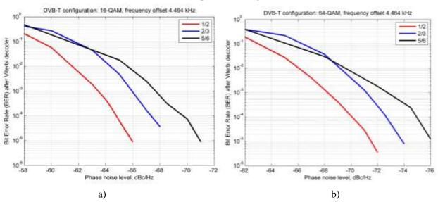
Figure 3 - Dependence of BER after Viterbi decoder from phase noise level in DVB-T system for 16-OAM (a) and 64-OAM (b) modulations and 4.464 kHz frequency offset
