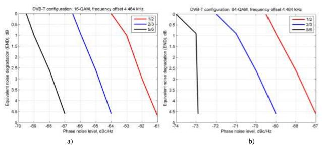
Figure 7 - Dependence of equivalent noise degradation value from phase noise level for 16-QAM (a) and 64-QAM (b) in DVB-T system
