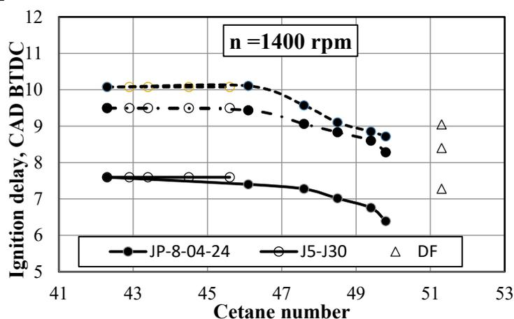
Fig. 1. Dependencies of ignition delay on the cetane number JP-8 fuel treated with CN improving additive and RME for engine loads of bmep = 0.104, 0.376 and 0.752 MPa at speed of 1400 rpm
