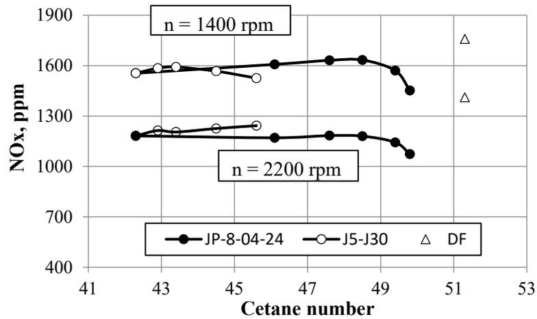
Fig. 3. The effect of CN improving agent and RME added to JP-8 fuel on maximum  $\text{NO}_x$  emission for full engine load and speeds of 1400 and 2200 rpm
