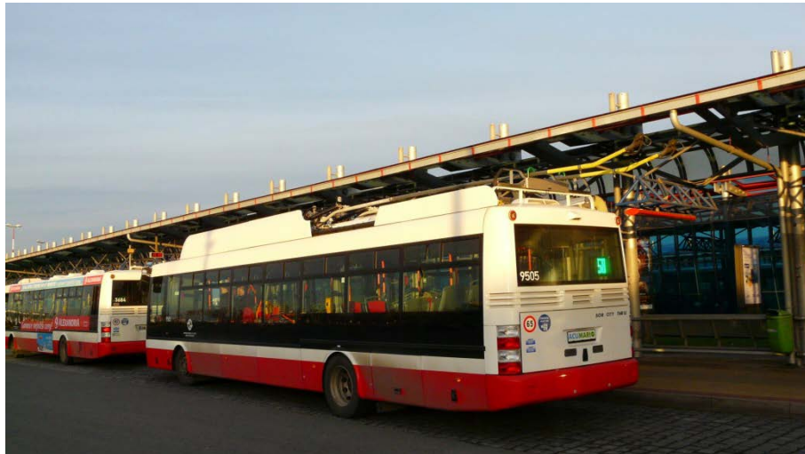
Fig. 5. Trolleybus SOR TNB 12 on Letňany terminous in autonomous drive mode
