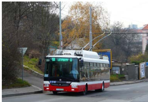
Fig. 4. Trolleybus SOR TNB 12 goes uphill on Prosecka street in Prague powered from the traction network
