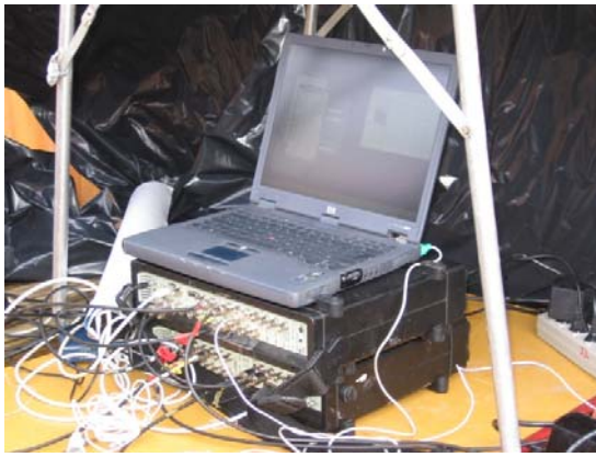
Fig. 8. Measurement devices (Bruel & Kjaer amplifiers and Noptel OY PSM200 laser device)
