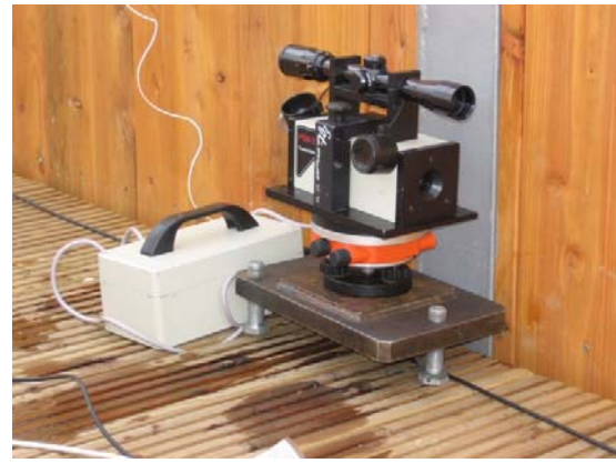
Fig. 8. Measurement devices (Bruel & Kjaer amplifiers and Noptel OY PSM200 laser device)
