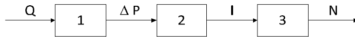
Fig. 4. Structural diagram of gas dynamical capillary flowmeter of small and micro flowrates of gas: 1 is a gas dynamical capillary flowrate transducer; 2 is a differential pressure gauge with a unified electrical analog output signal; 3 is a secondary device
