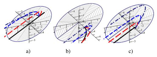
Fig. 4. The trajectories *r* (*t*) particles on rough inclined disc
