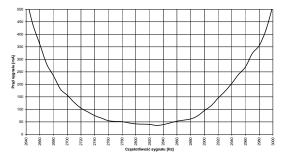
Fig. 7. Sensitivity features of MER111404/5 receiver in frequency function
