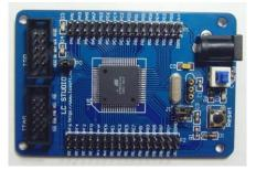
Figure 3 - Board with ATMega128
