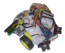
Figure 11 - Robot breadboard version
