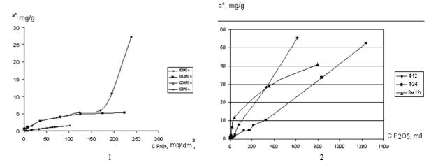
Fig. 3. Isotherms of phosphates adsorption: On natural zeolite (1), KH<sub>2</sub>PO<sub>4</sub> on synthetic zeolites (2)
