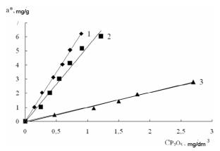
**Fig. 4.** Isotherms of phosphates, (KH<sub>2</sub>PO<sub>4</sub>) adsorption on natural zeolite (1), jointly with ammonium nitrogen (2), jointly with ammonium nitrogen and albumin (3)
