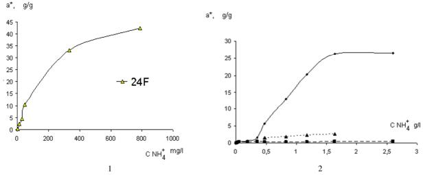
Fig. 2. Isotherms of ammonium adsorption on natural zeolite (1) on synthetic zeolite (2)
