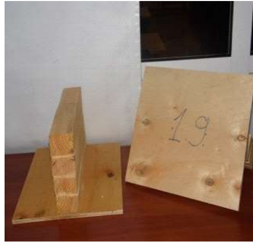
Figure 1 – Fragment of a Wooden Beam for Testing with Location of Thermocouples.
