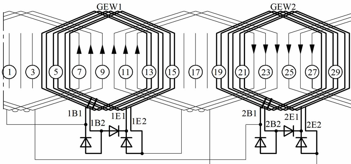
Fig.2. Winding with a periodically changing rotor structure distribution scheme
