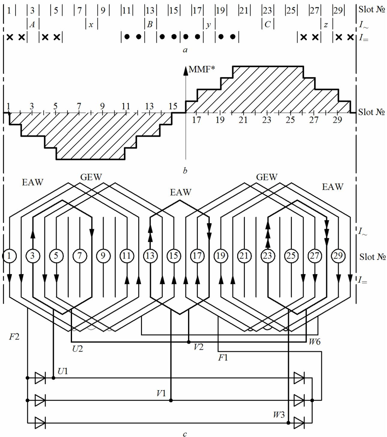
Fig.1. CCSG rotor winding scheme
