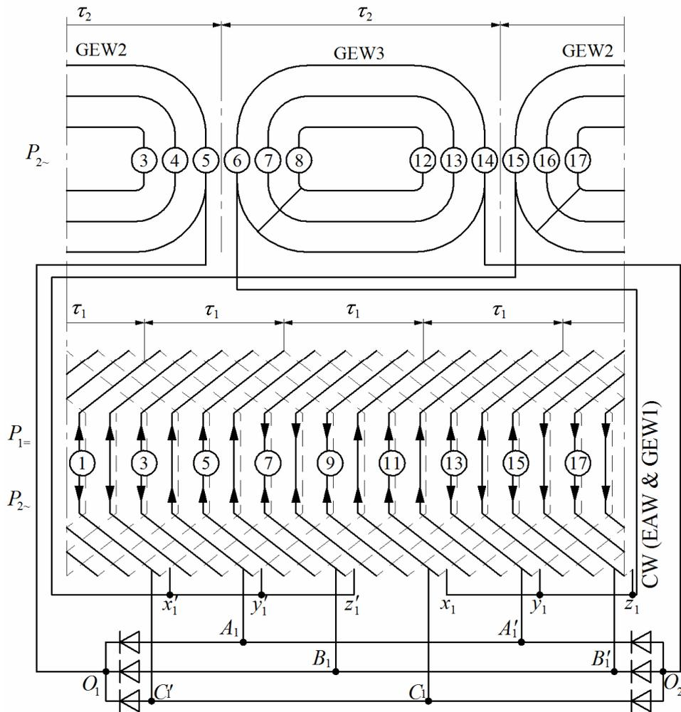
Fig. 3. Karavaev V.T. CCSG rotor combined winding distribution scheme
