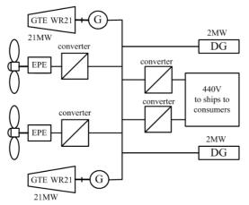
Fig. 2. Diagram of EU with complete electric propelling of Destroyer *Type* 45
