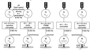
Fig. 1. Electric propulsion options
