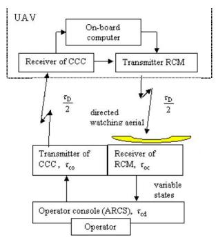
Simplified block diagram of the control system of UAV
