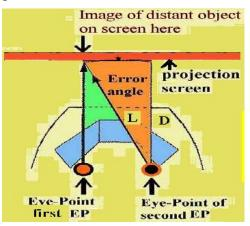
Fig. 5. An example of the layout of the operator and the EP relative to screen CS
