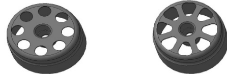
Fig. 3. Sensors with circle and triangle holes geometry
