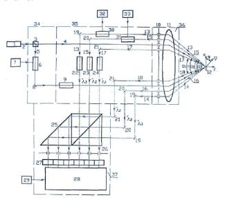
Fig. 3.Multiwavelength laser doppler anemometer (MLDA)
