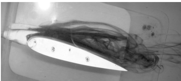
Fig. 2. A part of unsteady flow over the wing with vortex generator on the leading edge, \alpha = 15^\circ
