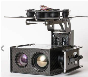
Fig. 6. A camera on gyro-stabilized platform
