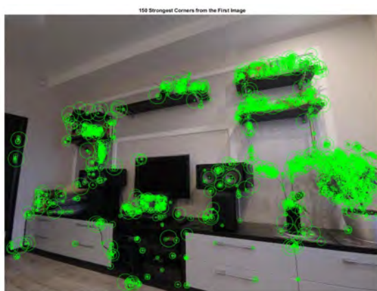
Fig. 16. Detected descriptors on the first image
