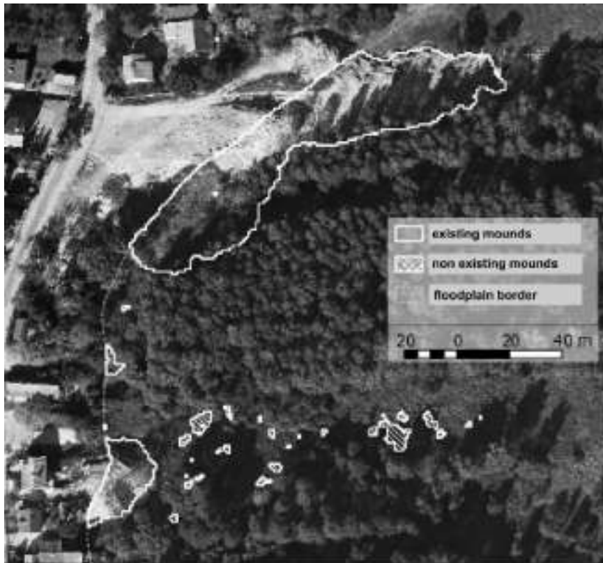
Fig. 3 – Mounds areas generated with the threshold value of +1 m (white line) corresponds to new mounds visible on the orthophotomap from 2011, additionally a group of generated artifact, non-existing mounds is visible
