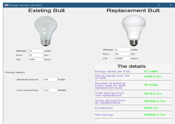
Fig. 2. The main program window for calculating the economic effect of modern lighting devices in enterprises
