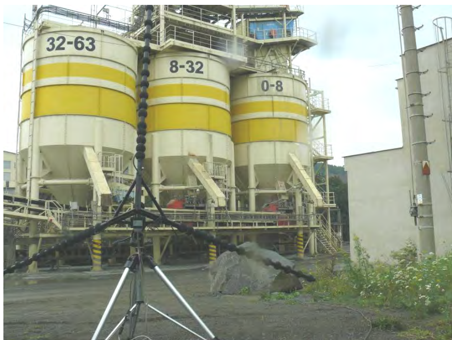
Fig. 8 Instaled acoustic camera by tanks in stone quarry
