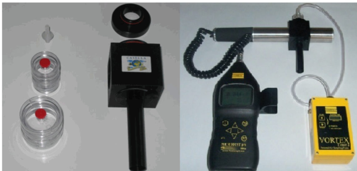
Fig. 2 Adapter for gravimetric method
