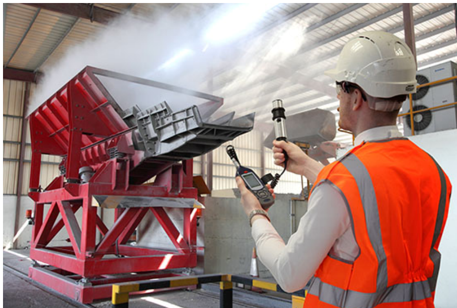
Fig. 3 Real-time dust monitoring instrument in practice
